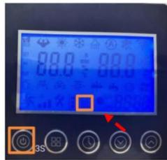
**7.2.3 Step1 (Lock):**
